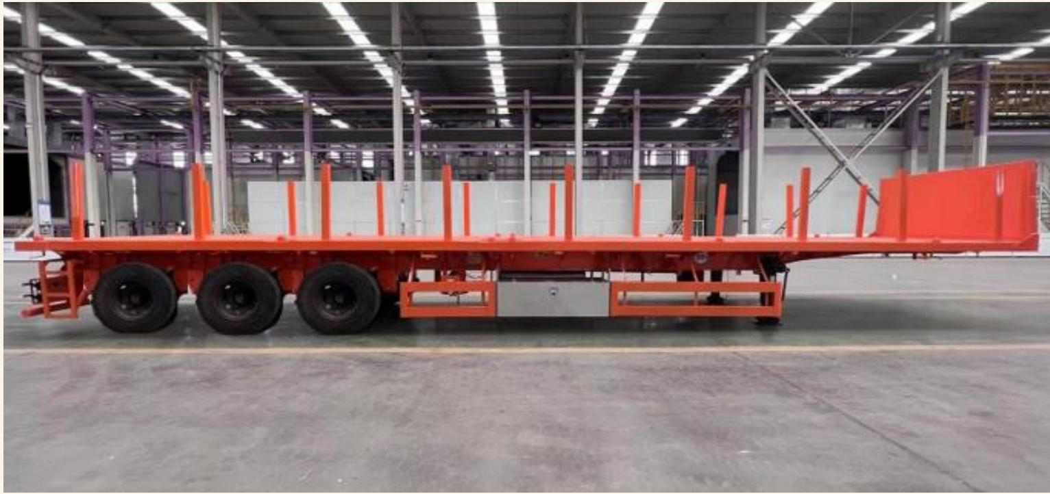
**Flatbed semi trailer** is one of our main product. This series of semi trailers use through beam structure, where frame structure has flat type. It has the characteristics of high integral strength, small weight, elegant appearance, strong loading capacity, and reliable operation.
