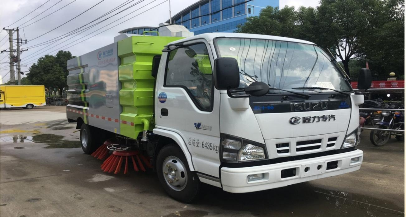
A road sweeping machine is a specialized vehicle designed to efficiently clean and sweep roads, streets, and other paved surfaces. It utilizes brushes, suction systems, and water sprayers to remove dirt, debris, and other pollutants from the road surface.
