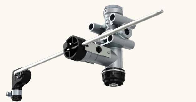
**Height limitation:** The levelling valves 464 006 100 0, 464 006 101 0 and 464 006 201 0 have an additional 3/2-way valve that closes as of a certain adjustable lever angle and switches to a venting function upon actuating the lever again. This "Height limitation" prevents the vehicle from being raised above a permitted level with the rotary slide valve.
