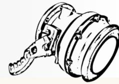
API adapter valve is installed on one side of the bottom the tanker, with the design of quick connecting structure. Interface dimension is designed according to the API RP1004 standard. This is an important component of the bottom loading system to get quick detachment without leakage. It is much more safe and reliable when doing the work of loading and unloading. It is suitable for unloading corrosive chemical materials.
