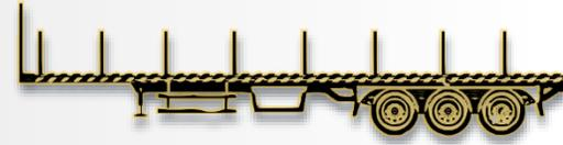
**3 Axel with Max Loading 12 ton for each Axel with Air Suspension system**
