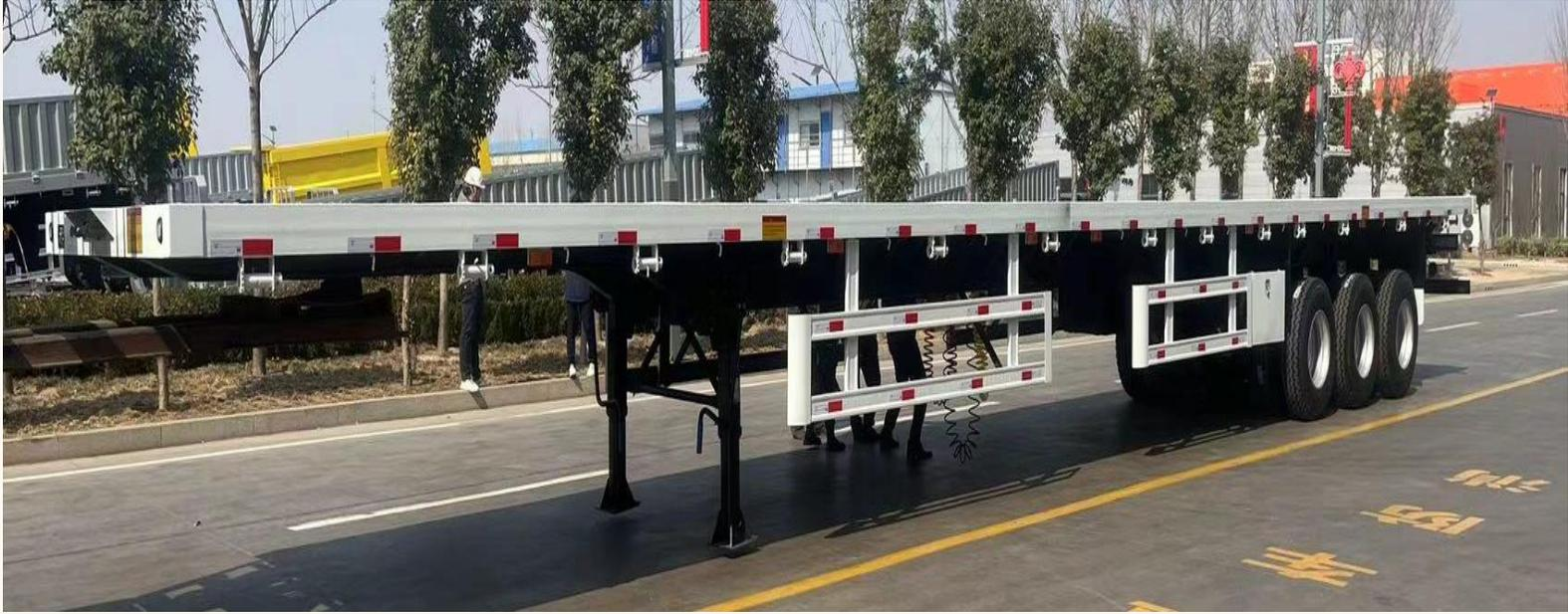
Flatbed semi trailer is one of our main product. This series of semi trailers use through beam structure, where frame structure has flat type. It has the characteristics of high integral strength, small weight, elegant appearance, strong loading capacity, and reliable operation.
