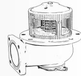
Bottom Valve is install on the bottom of the tanker with the disc sealed inside it . Valve body with self-cut groove. When in the event of accidental damage, the external housing will break away from the self -cut groove, keeping the connection to the valve tank mounting flange ,leaving the bottom valve sealing mechanism within the tank compartment intact,efficiently protecting the tanker from leakage ,ensuring the safety of transportation.
