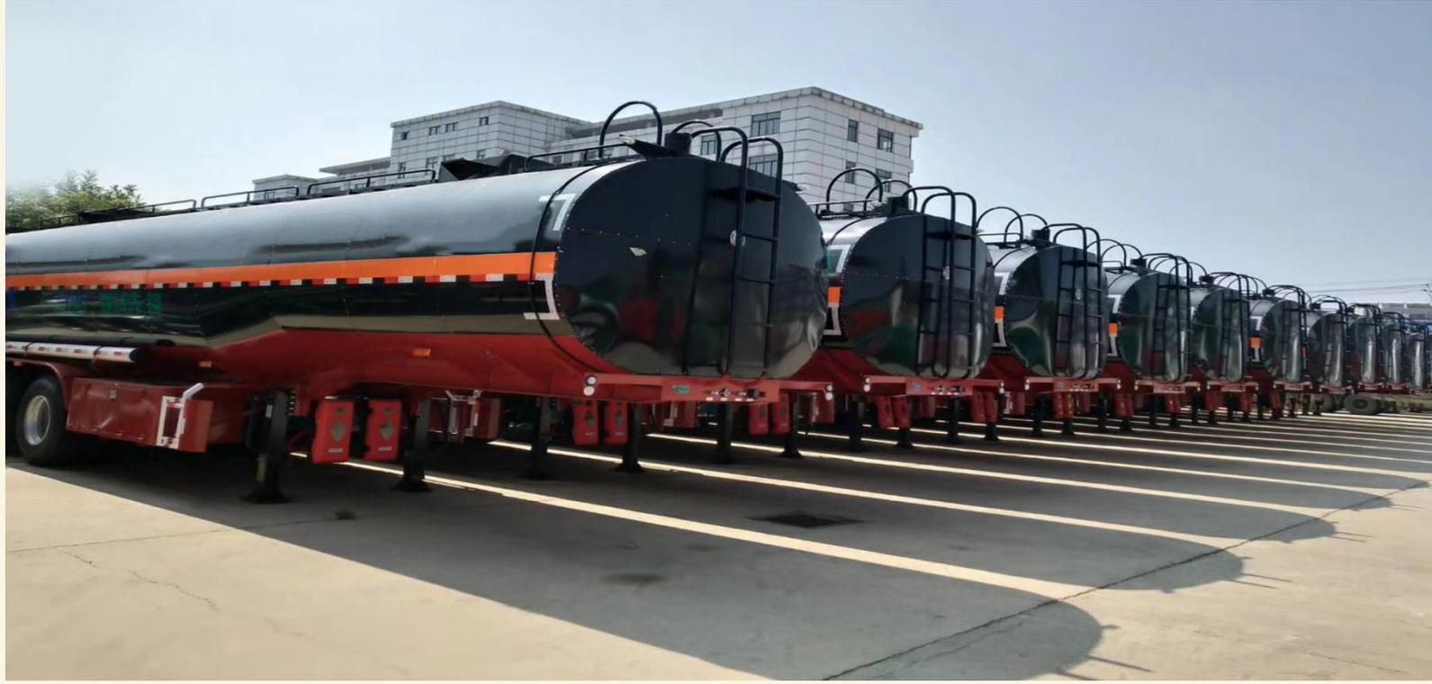
Asphalt transport semi-trailer is one of our products. Used for transporting asphalt material. The tank body is made of bright aluminum with a thermal insulation layer of glass wool up to 50mm and with two heating path design. The trailer has the characteristics of high integrated strength, elegant appearance, strong loading capacity and reliable operation.
