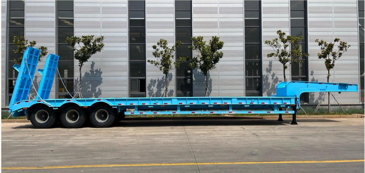
Lowbed semi trailer is one of our main product. This series of semi trailers use through beam structure, where frame structure has Goose neck type. It has the characteristics of high integral strength, small weight, elegant appearance, strong loading capacity, and reliable operation.
