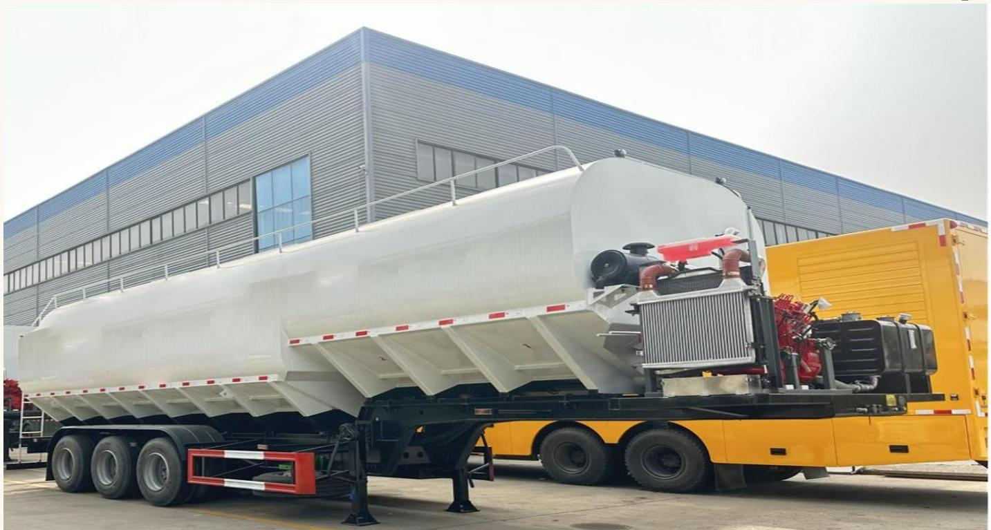
The poultry feed semi-trailer with a capacity of 50 cubic meters is considered an effective and reliable option in the agricultural sector, featuring a strong and secure front. This system excels in efficiently loading and transporting feed, contributing to improved livestock management.
