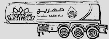
**3 Axel with Max Loading 12 ton for each Axel
