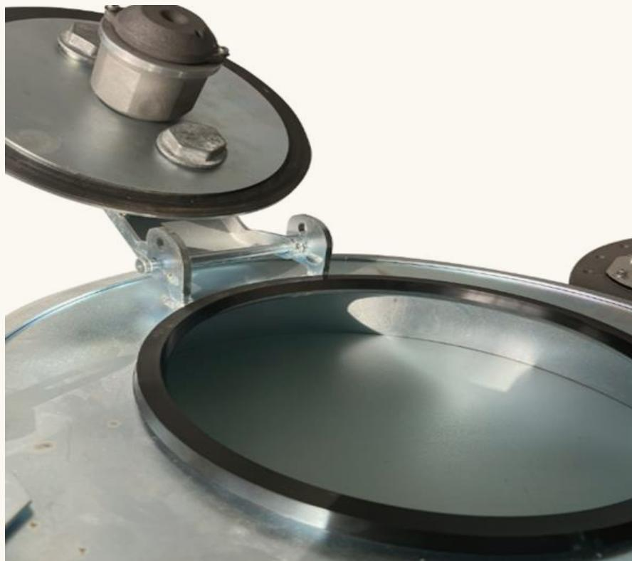
The first type is a manhole cover without a breathing valve. It is suitable for natural exhaust and does not require high sealing. It prevents high-temperature tanks from holding air and is used for filling water or checking internal functions.
