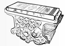
It is normal to mount the TEBS G2.2 Brake Module with the mounting studs towards the rear of the vehicle with the brake actuators on the left side supplied by Port 22 and on the right side by Port 21 (the ports closest to the actuators). However, it is permissible to mount the module with the mounting studs towards the front of the vehicle providing that the orientation is changed in under the “Information” tab and “Change configuration”.
