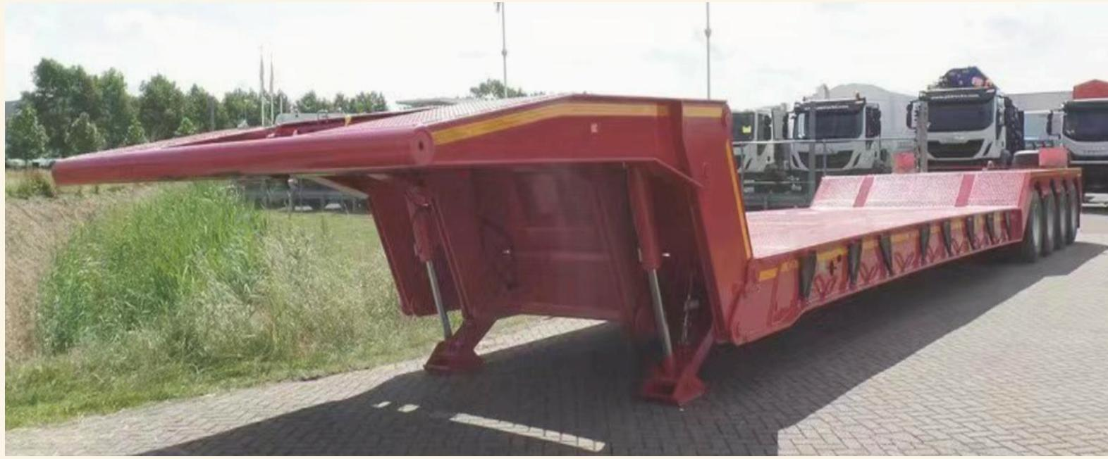
**Lowbed semi trailer** is one of our main products. This series of semi trailers use through beam structure, where frame structure has Goose neck type. It has the characteristics of high integral strength, small weight, elegant appearance, strong loading capacity, and reliable operation.
