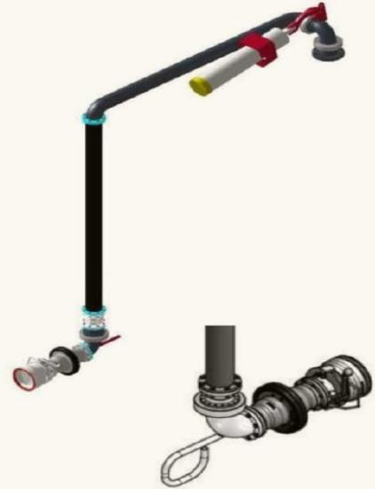
The HG-type bottom-mounted crane hose system is composed of a "liquid loading and unloading arm "and a "quick-release flange-type separation valve.“ It is used for transferring liquid media between loading platforms and tankers to complete the loading operation. Key components include the crane hose kit, dry valve, and breakaway valve.
