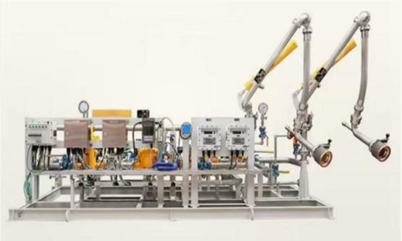
The oil unloading device uses 3 independent motors and pumps to load and unload three kinds of oil products such as diesel and gasoline respectively. It is closed, portable and operated by a mobile crane tube. It consists of a gas system and a control system. The configuration of the unloading device is determined according to customer needs. In areas with harsh conditions, the configuration should be simplified as much as possible to ensure equipment stability.
