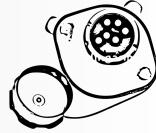
API Optic socket is one part of whole vehicle mounted overfill prevention control system and grounding system. API Compatible Optic Socket is installed on the side of tank truck, API optic socket transfers static signal and overflow signal. API overfill socket is used for interlock air break systems, it can ensure vapor vents are open before loading fuel.
