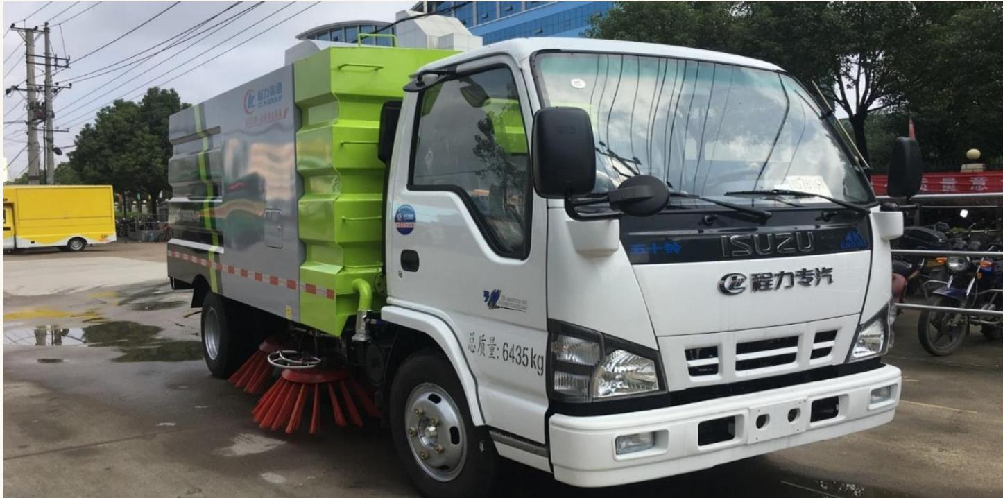
A road sweeping machine is a specialized vehicle designed to efficiently clean and sweep roads, streets, and other paved surfaces. It utilizes brushes, suction systems, and water sprayers to remove dirt, debris, and other pollutants from the road surface.
