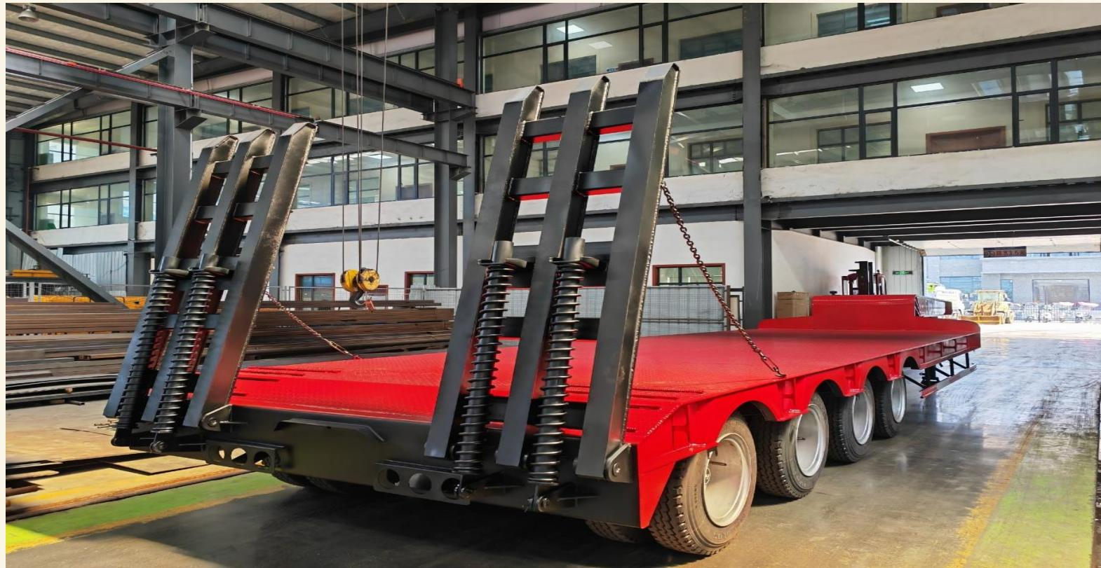
**Lowbed semi trailer is one of our main products. This series of semi-trailers uses cross-beam structure, the frame structure is neck type, and has the characteristics of high integral strength, small weight, elegant appearance, strong loading capacity, and reliable operation.**
