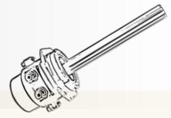
Anti- overflow probe is mainly used in the tanker, tank material add conditions, when charging excessive internal signal transmission terminal, and prompted the installation platform to stop charging, so as to ensure the safety of the installation. The anti-overflow probe and the overflow socket and the earth stud together form an antistatic system.
